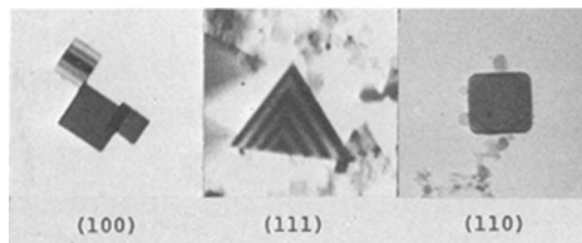
Figure 8 Three typical types of ultrafine TiN particles found in this study.
